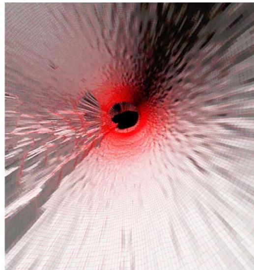
3D visualization of a fully flooded zero-visibility situation in a vertical pipe. Note the heavy rag buildup on the rungs of the access ladder on the left.
